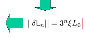
The current sharing increases with the coupling between the filaments  $1/\epsilon_0$  and the number of nesting level n.
